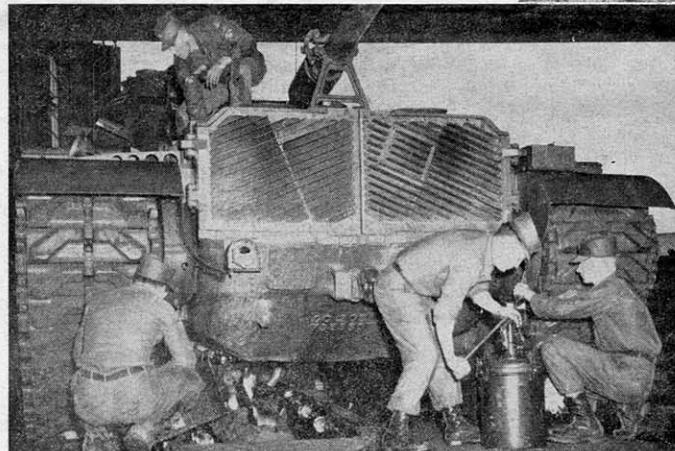
Deprocessing an M60 tank (left) before issuing it to a unit, men of the 122d Ord Bn drain preservatives from the armored vehicle. The tank is then given a complete lubrication. Deprocessing new vehicles is one of the routine operations performed by the ordnance battalion. (Below) Among the support and services offered by the 503d MP Co is directing traffic during training at Grafenwoehr.
